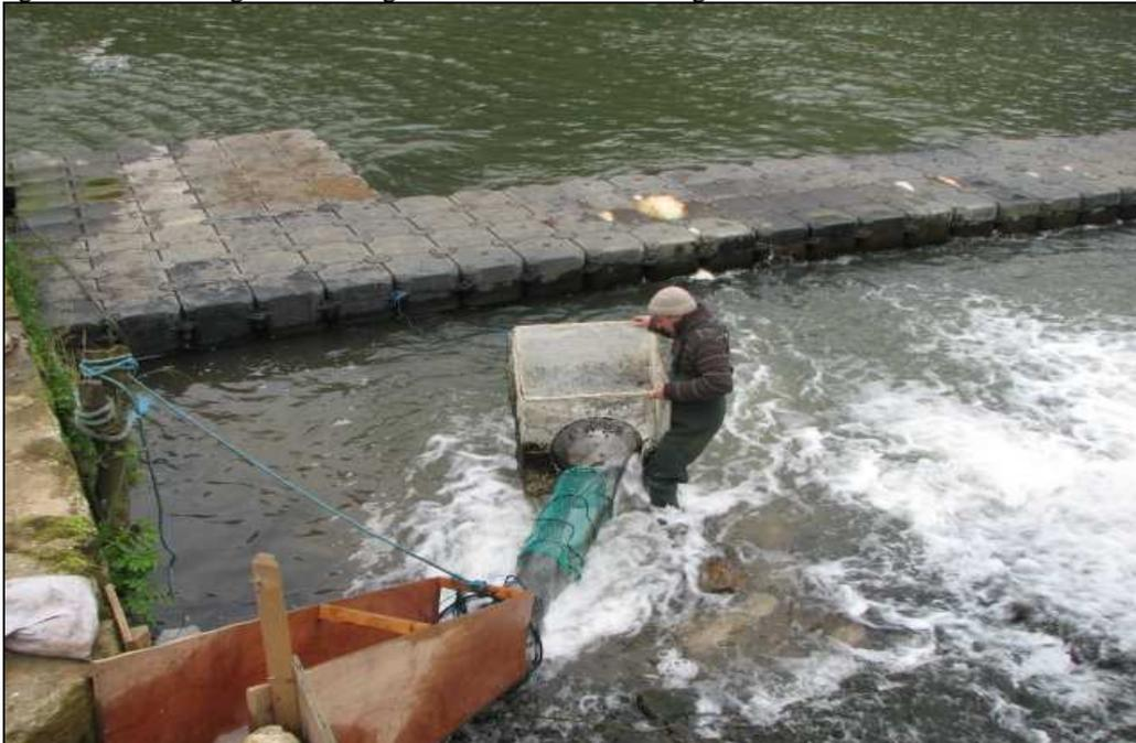
**Figure 3:** photograph illustrating the chute and holding box.
